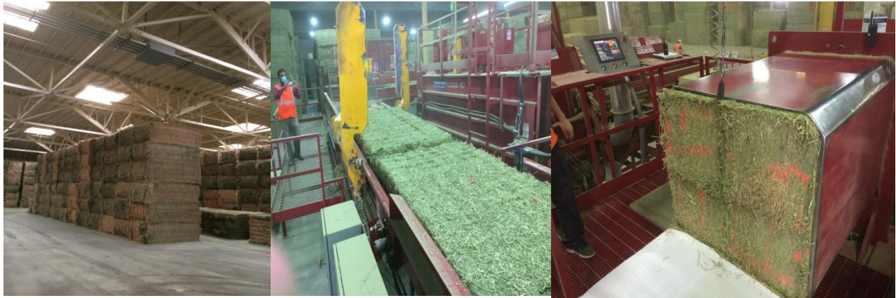
Figure 1. Single compressed, baled hay (left) is often cut and re-packaged to a more compressed bale for long-distance transport. These bales present challenges for sampling.
